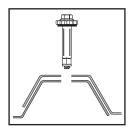
Insert Fab-Lok into a 5/16" to 11/32" diameter hole
