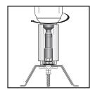
Use the Dewalt screwgun or other drive tool to expand the Fab-Lok fastener until the clamping tines are tight against the backside of the material being fastened. The Fab-Lok fastener is fully seated when the tool begins to ratchet and the fastener stops turning. Installation should be slow and controlled, with a maximum speed of 1000 rpm.
