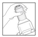
Slide the Fab-Lok setting tool over the nose of a DEWALT versa-clutch screw gun and tighten the set screw with the included hex key. The torque setting of the tool should be adjusted to ensure a proper installation without overdriving.
