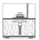
Can be used in blind applications, such as attaching to insulated metal panels.
