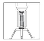
Secure the head of the Fab-Lok fastener with a Fab-Lok setting tool on a dewalt versa-clutch screw gun or using 5/16" nut driver in combination with a 5/8" box wrench or vice grip type tool to hold the collar of the aluminum sleeve of the
